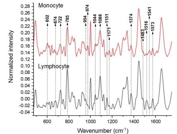
Fig.9 : Raman spectra of monocyte and lymphocyte with Raman signature showing cell differences.
