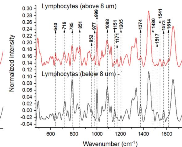
Fig.11 : Raman spectra of lymphocyte (above 8 μm) and lymphocyte (below 8 μm) with Raman peaks
