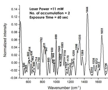
Fig.5 : Raman spectrum of an optically trapped Neutrophil
