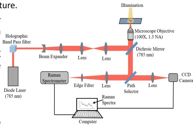
Fig 1. Schematic of Raman Tweezers experimental setup
