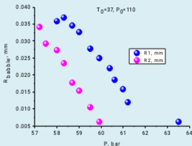
Fig. 2. The characteristic bubble radii versus the current pressure.
