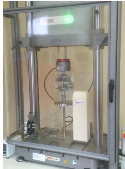
Fig.3. Device for multi-cycle loads Instron Electropuls E3000
