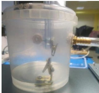
Fig.2. Process of sample testing in physiological environment at a temperature 37°C
