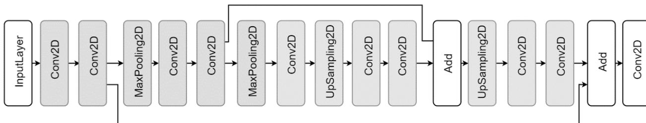
Figure 5 – CNN2 architecture
