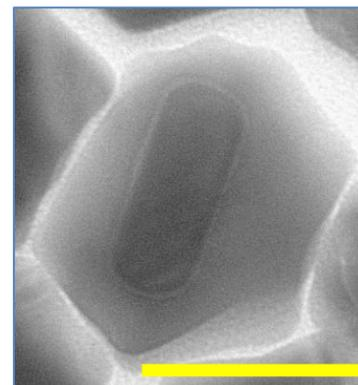
Shape of the nanocore significantly affects the signal intensity and the SERS enhancement factor for uncoated and GERTs nanoparticles, and maximum increase in the SERS signal and the enhancement factor was observed for nanorods.
