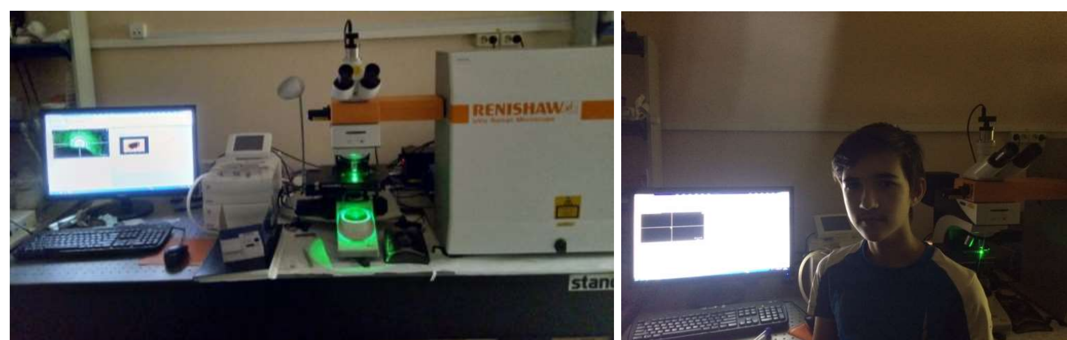
Fig. 2 Raman spectroscopy allows to see different functional groups of molecules: C-C, C=C и C-CH3 bonds in carotenoids.
