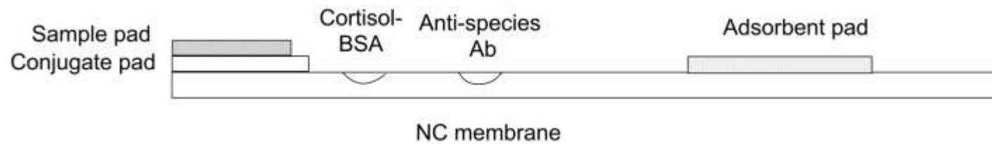
To make test-strips, we use NC membranes type CNPF-SN-12-L2-H50, sample pad type GFB-R7L, adsorbent pad type AP 045, conjugate pad type PT-R7. All from mdi Advanced Microdevices Pvt. Ltd, India.
