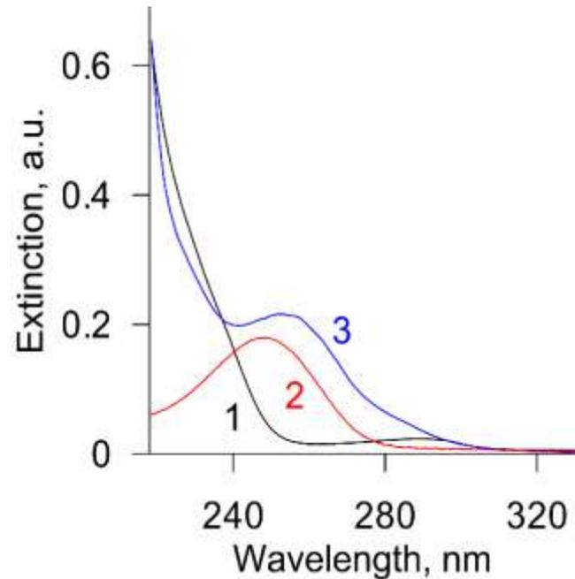
Figure. 1. Extinction spectra of BSA (1), cortisol (2), cortisol-BSA complex (3). The shift in the absorption maximum from 248 nm to 251 nm is associated with the chemical modification of cortisol, with its presence in a bound state.
