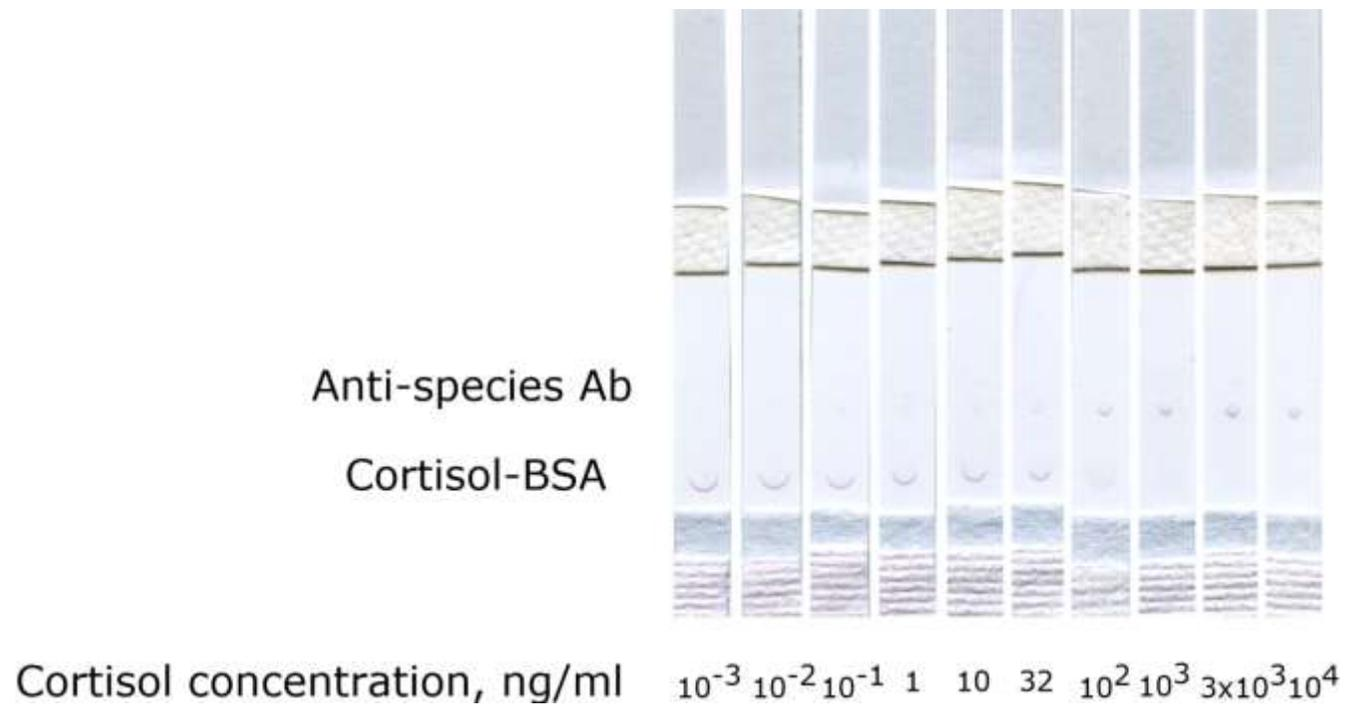
STEP 6. Digitize test-strips and make a calibration curve.
