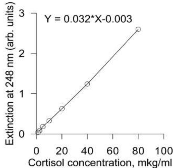
Figure. 2. A calibration graph of the dependence of the absorption of solutions of cortisol with a concentration of 1.25 to 80  $\mu\text{g} / \text{ml}$  from concentration at 248 nm. An approximating line equation:  $Y = 0.032 * X - 0.003$ .
