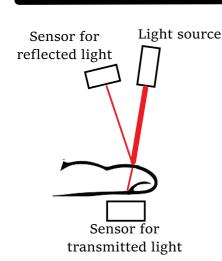
This laboratory model of a combined optical sensor and the corresponding software allows non-invasive monitoring of the liver functional reserves
