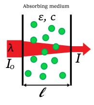
Optical densitometry is based on Bouguer-Beer-Lambert law. Increase of the optical density of the medium decreases light transmission.
