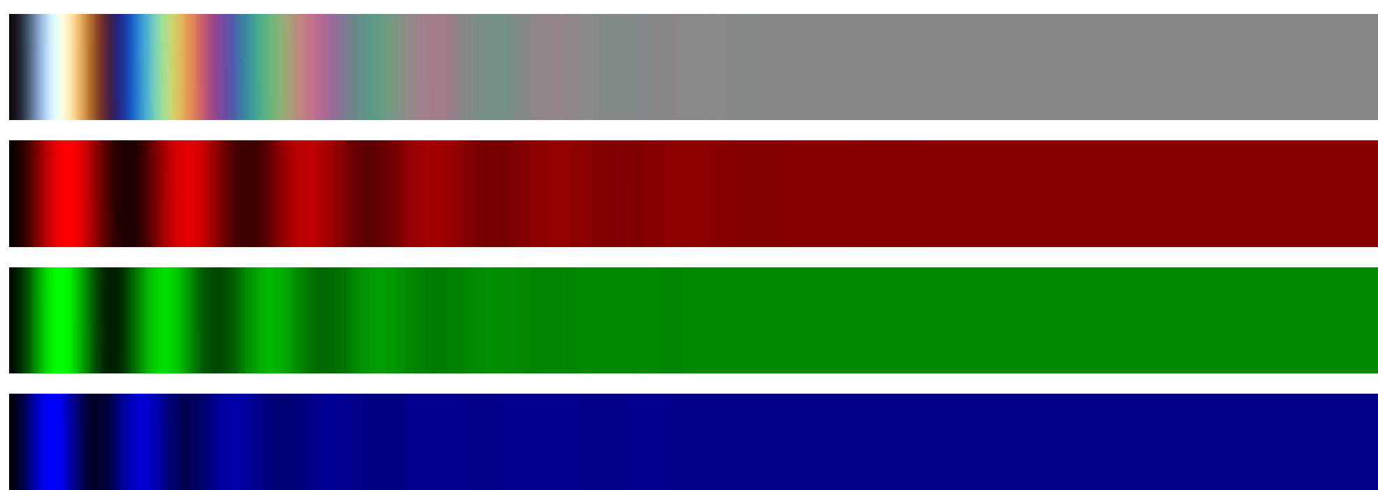
Fig.4. Influence of the width of the frequency spectrum of the interfering wave fields on decorrelation of the fields and the visibility of interference fringes
