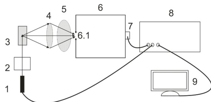
Fig. 1. Experimental setup. 1 - laser, 2 - Glan prism, 3 - cuvette with solution, 4 - lens, 5 - polarizer, 6 - monochromator, 6.1 - input slit of the monochromator, 7 - photomultiplier, 8 - TCSPC module, 9 - computer.
