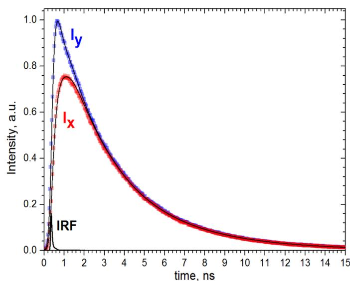
Fig. 2. Polarized fluorescence decay signals of FAD in aqueous solution at 530 nm.  $t = 0$  is the excitation time. Symbols denote experimental data and solid curves are fits obtained with due regard to an instrument response function (IRF). The decay curves  $I_x$  and  $I_y$  are intensities of the horizontally and vertically polarized fluorescence components. The IRF shown in the left-down side has a full width at half maximum of about 320 ps.
