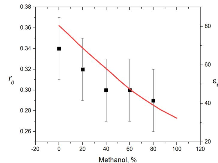
Fig. 5. FAD fluorescence anisotropy  $r_0$  as function of MeOH concentration. Red line represents the dependence of relative dielectric permittivity  $\epsilon_r$  of the solution on methanol concentration.
