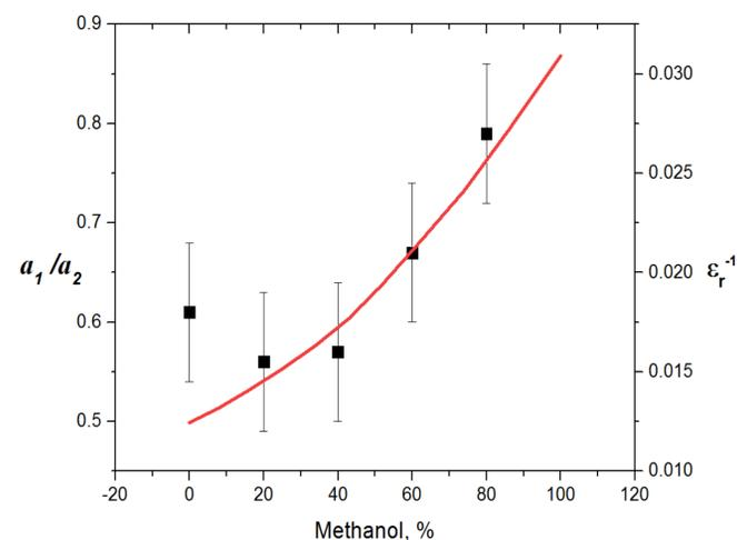
Fig. 4. Weighting coefficients ratio  $a_1/a_2$  as function of methanol concentration. Red line shows the inverse dependence of relative dielectric permittivity  $\epsilon_r$  on MeOH concentration.
