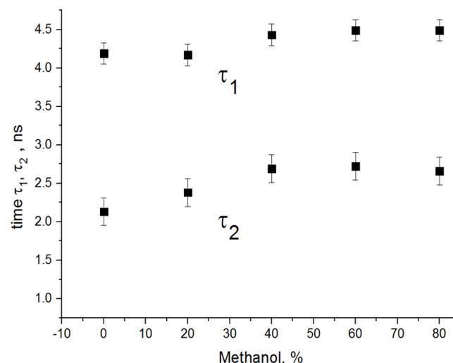
Fig. 3. FAD fluorescence decay times  $\tau_1$  and  $\tau_2$  as function of methanol concentration.
