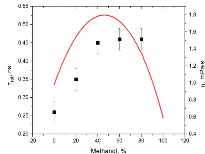
Fig. 6. FAD rotational diffusion time as function of MeOH concentration. Red curve presents solution viscosity as function of MeOH concentration.
