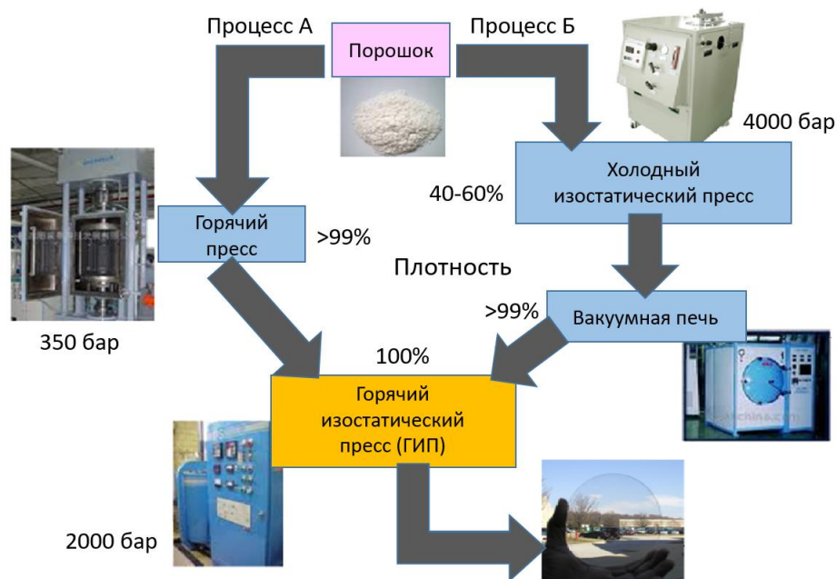
Fig. 1. Scheme for obtaining highly transparent oxide optical ceramics.
