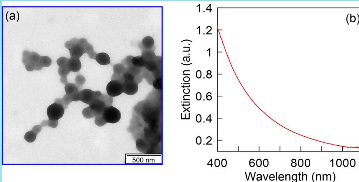
**Figure 2.** TEM image (a) and extinction spectrum (b) of synthesized albumin nanoparticles.
