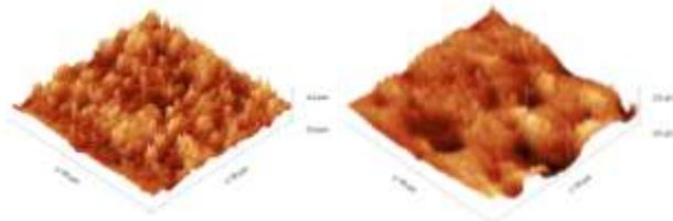
Atomic force microscopy images of the surface of thin hydrogel plates of chitosan L- and D-aspartates
