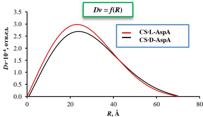
Functions of volumetric size distribution of scattering domains for hydrogel plates based on chitosan L- and D-aspartates
