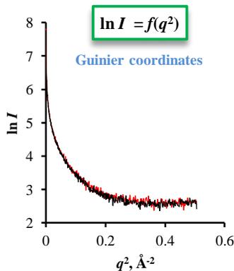
Small-angle X-ray scattering curves for hydrogel plates based on chitosan L- and D-aspartates
