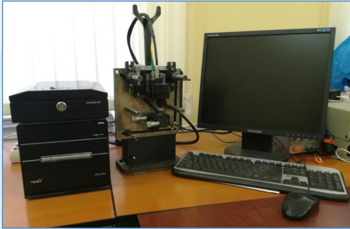
The Spectral Radar OCT System OCP930SR 022 (Thorlabs Inc., United States) with a wavelength of 930 nm
