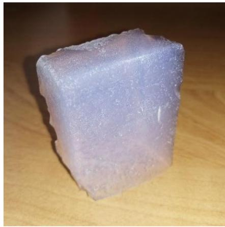
**Figure 1:** the example of silica aerogel
